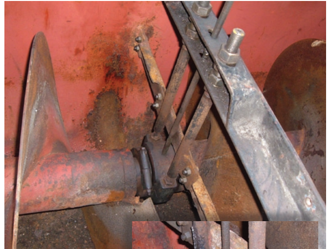
Screw conveyor equipped with a troublesome plain bearing before conversion
