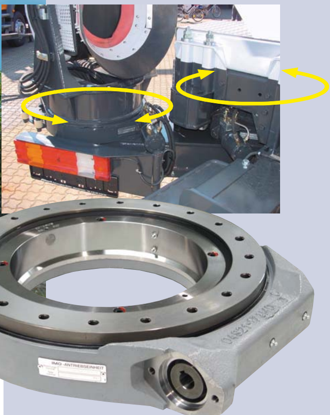
Cement mixer equipped with a conveyor belt with a length of 16.5 m, which is rotated with two WD-LC 0419 ; the considerable length of the belt leads to high tilting moments. Therefore a double row design with a reinforced housing is used.
