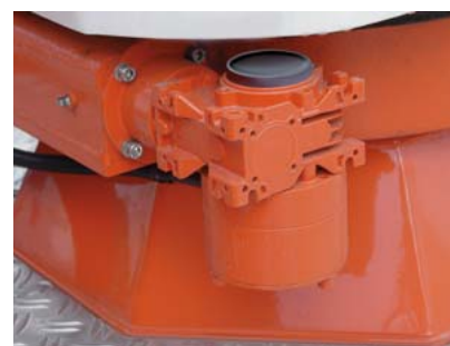
WD-L 0343 with the attached potentiometer, used in manlift systems
