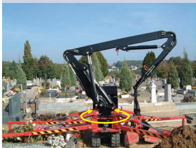
Cemetery excavator with the IMO Slew Drive WD-L 0343 .
