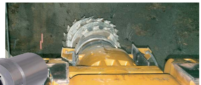
Slew Drive SP-HC 0698 with hydraulic motors and gear boxes for turning an excavator boom , part of a cutter bar of a tunnel boring machine.
