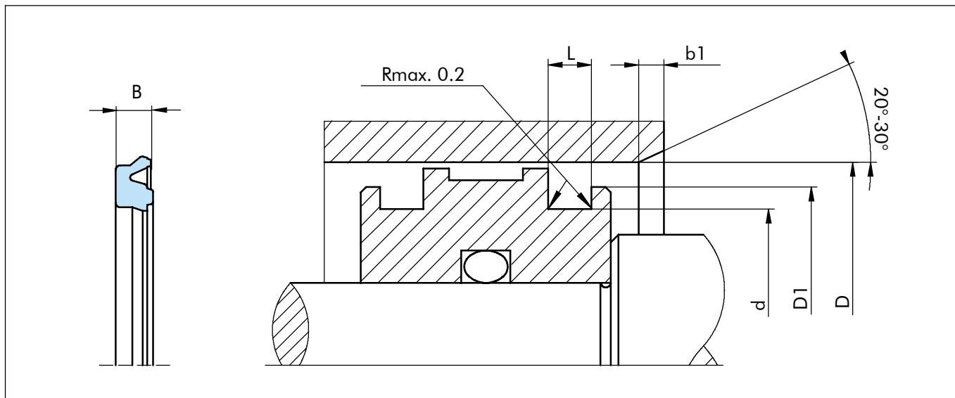
Figure 6 Installation drawing
