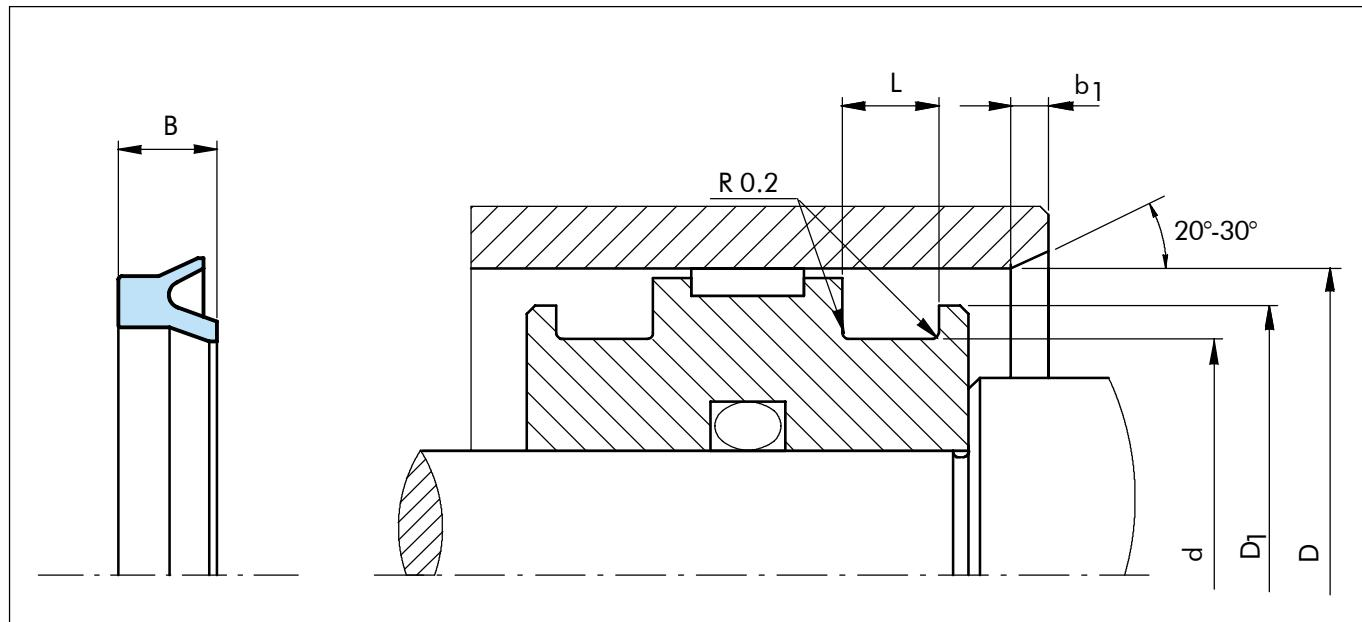
Figure 7 Installation drawing
