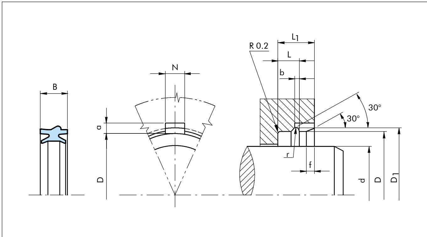
Figure 15 Installation drawing
