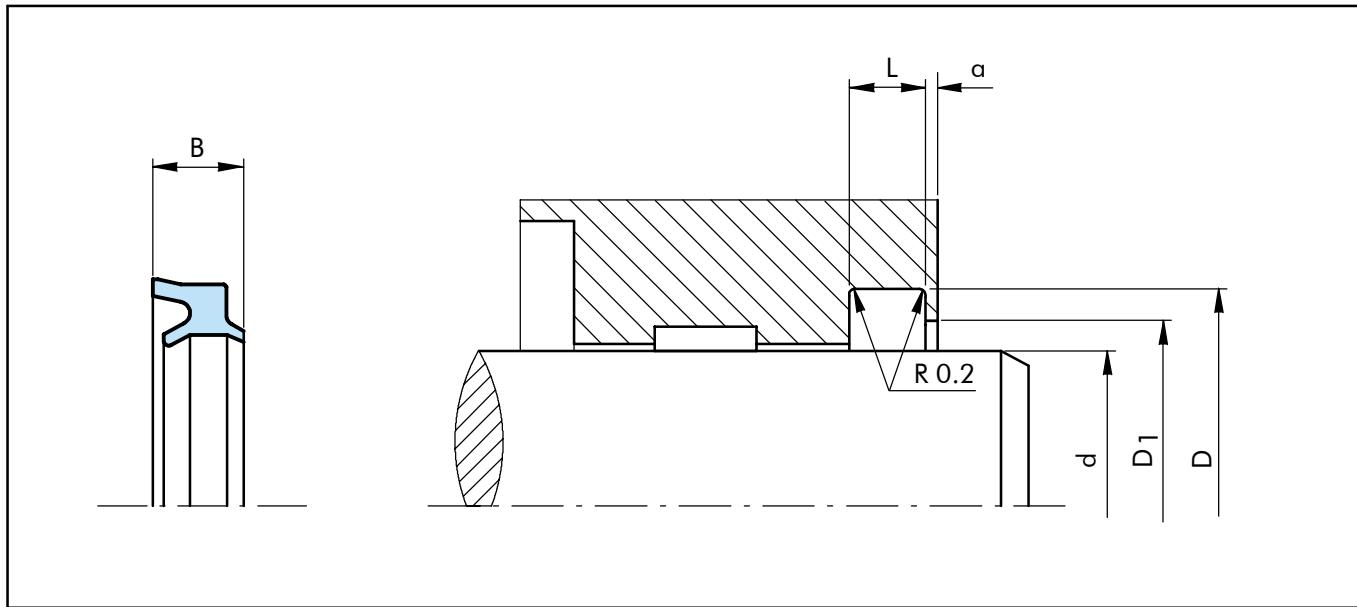
Figure 13 Installation drawing
