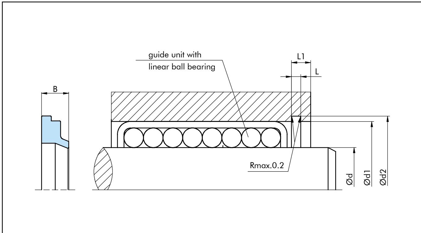
Figure 18 Installation drawing
