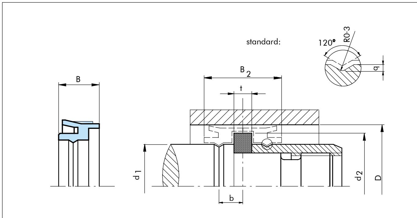
Figure 8 Installation drawing
