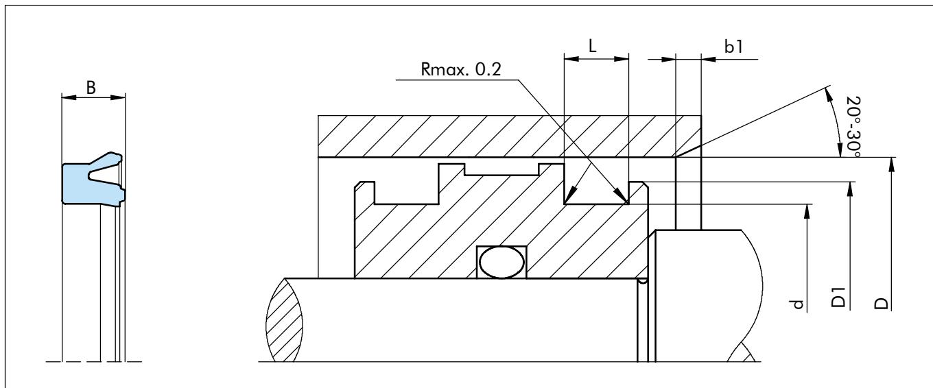
Figure 5 Installation drawing
