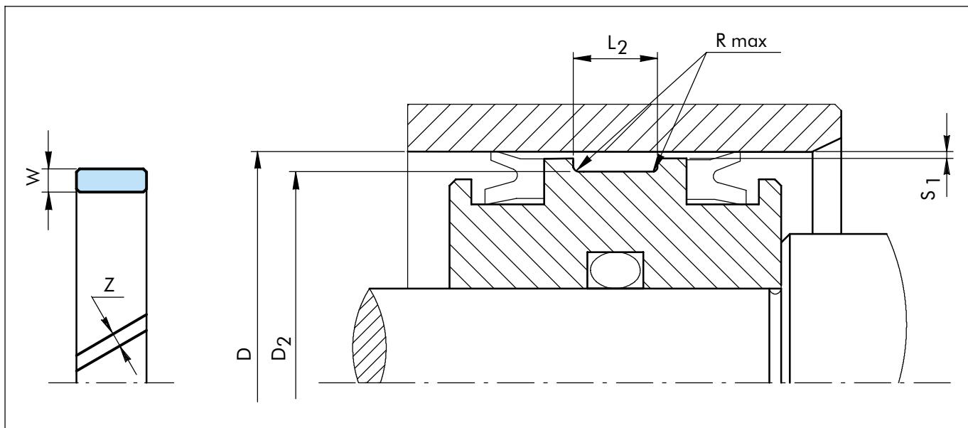
Figure 23 Installation drawing
