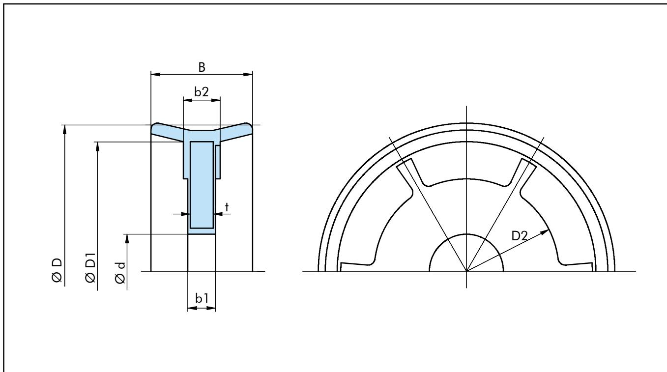
Figure 11 Installation dimensions
