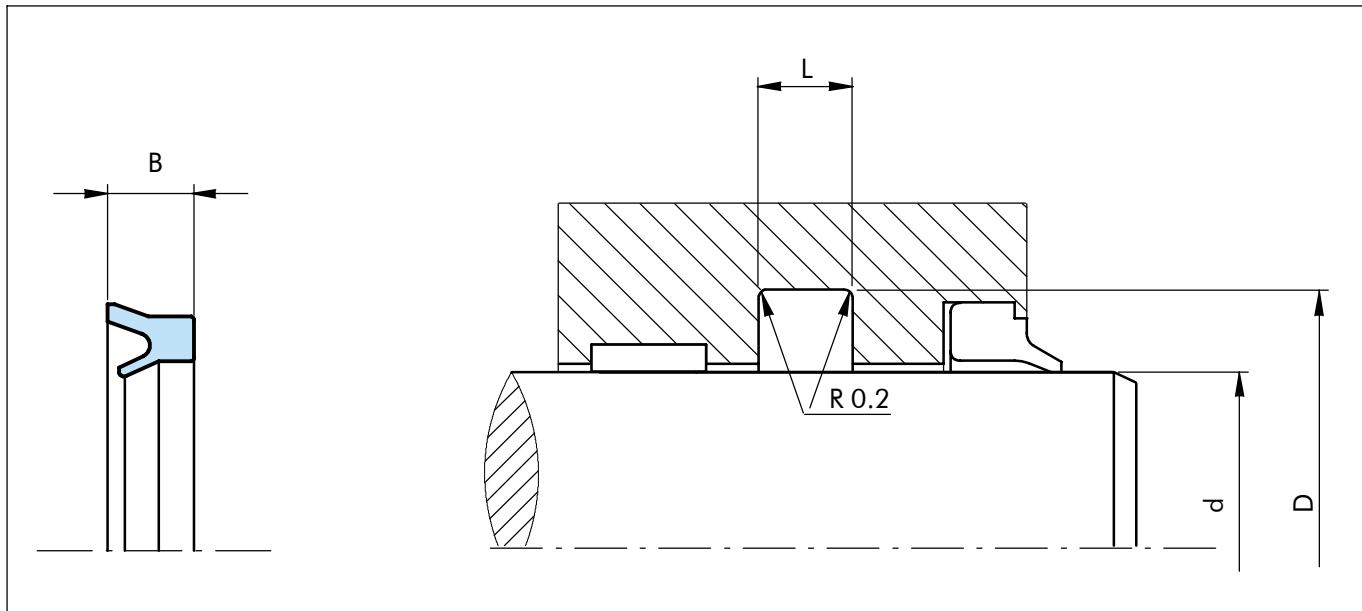
Figure 2 Installation drawing
