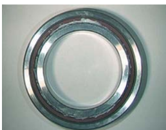
Photo. 6.1 Filling grease into angular contact ball bearing
