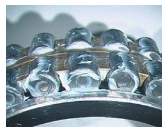
Photo. 6.2 Filling grease into cylindrical roller bearing
