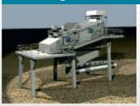
To extract the under-sized materials from the crushed ore, two successive screening techniques are used:
