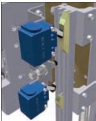
Mechanical and inductive micro-switches on MC series.
