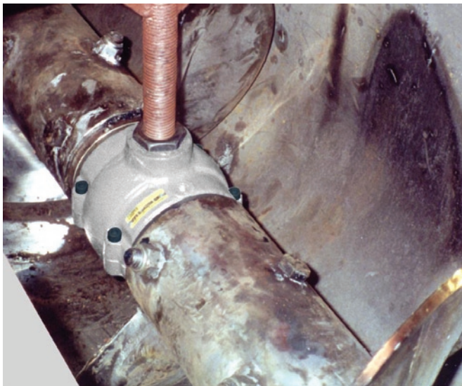
Typical hanger on a screw conveyor
