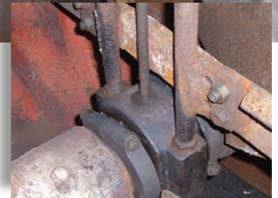
Screw conveyor equipped with a troublesome plain bearing before conversion
