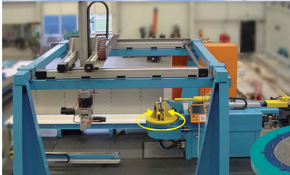
SP-Slew Drives are used in automation systems. Picture: Slew Drive SP-LE 0641 with three-phase electrical motor and spur gearbox.
