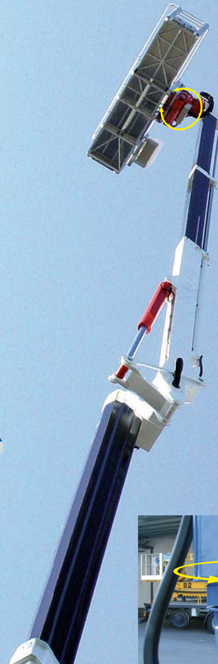
This working platform with a height of 35 m uses two IMO Slewling Rings on a synchronous rotating turntable which are driven by an IMO WD-HC 0146 Slew Drive.
