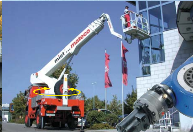
This working platform with a height of 35 m uses two IMO Slewling Rings on a synchronous rotating turntable which are driven by an IMO WD-HC 0146 Slew Drive.
