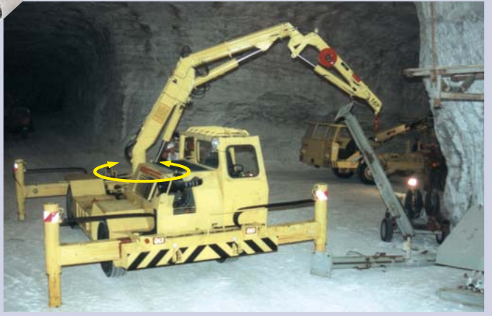
Working in aggressive environmental conditions, the Slew Drive WD-HC 0373 is adapted for the use by a crane in a salt mine . Brakes ensure position holding at extreme crane decline.
