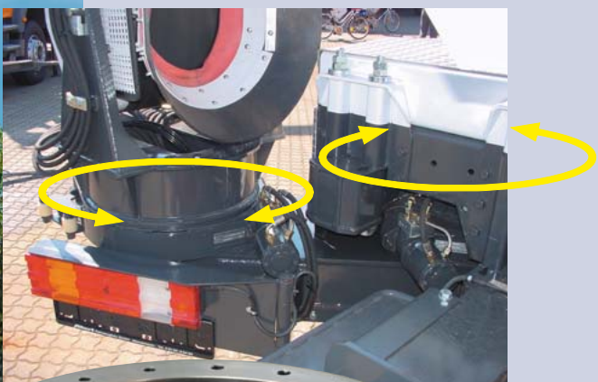
Cement mixer equipped with a conveyor belt with a length of 16.5 m, which is rotated with two WD-LC 0419 ; the considerable length of the belt leads to high tilting moments. Therefore a double row design with a reinforced housing is used.
