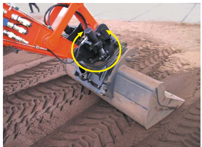
This rotation and tilting device of a front loader uses an IMO Slew Drive, model WD-LC 0419 with twin motors (double the torque).
