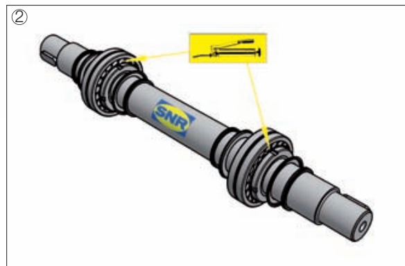
② Clamp the shaft horizontally (protect the shaft against damage in the area of the clamping). The internal contact washers and V-rings are slid onto the shaft first. The sequence and arrangement of the sealing elements is crucial to ensure correct mounting.
