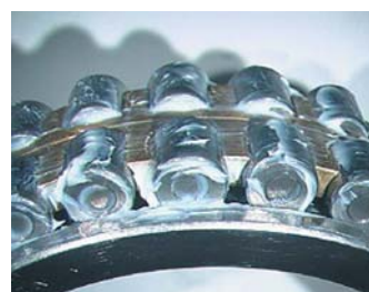
Photo. 6.2 Filling grease into cylindrical roller bearing
