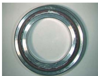
Photo. 6.1 Filling grease into angular contact ball bearing
