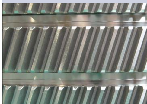
External helical gear, normalized
