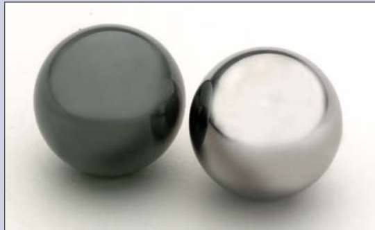
Ceramic and steel balls
