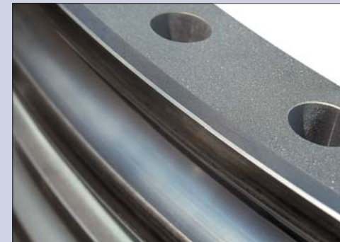
Zinc-coated surface (flame-sprayed)
