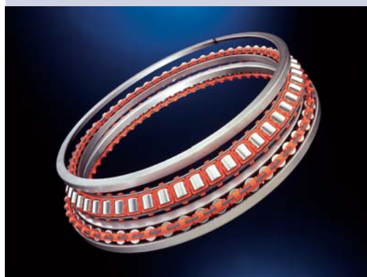
Double Row Angular Contact Cylindrical Roller Slewing Ring for the chain wheel of a tracklaying vehicle. These separable rings are not self-supporting but integrated into the housing as individual parts by the customer.
