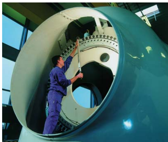
Assembly of a Blade Bearing on the hub.
