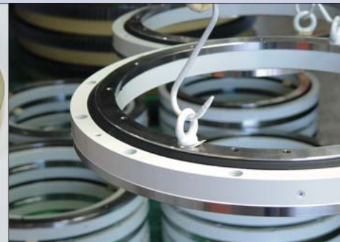
Priming and multi-coat painting
