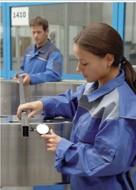
Acceptance testing of a Roller Slewing Ring.
