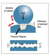
The service life of the bearing is directly related to the efficiency of the lubricant film, which depends on:
