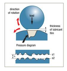
The service life of the bearing is directly related to the efficiency of the lubricant film, which depends on:
