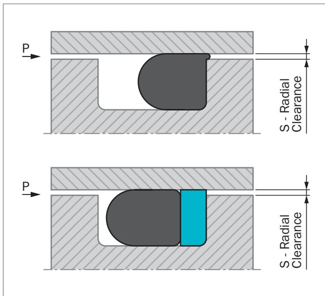
Figure 41: O-Ring installation with and without Back-up Ring
