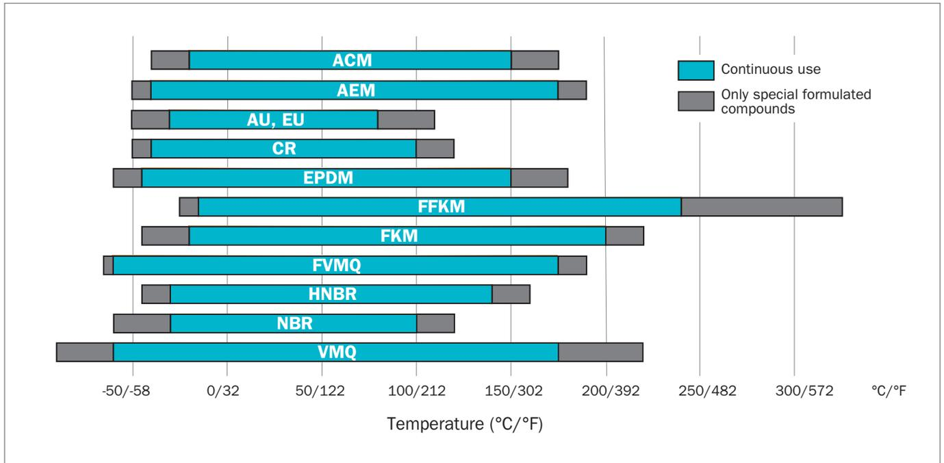
Figure 4: Temperature ranges of various elastomers
