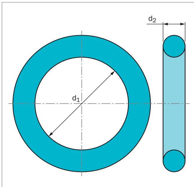
Figure 1: O-Ring dimensioning
