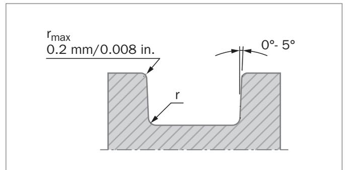
Figure 26: Groove specifications
