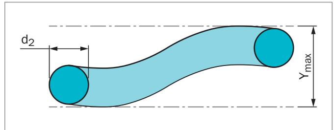
Figure 28: Flatness tolerance  $Y_{max}$
