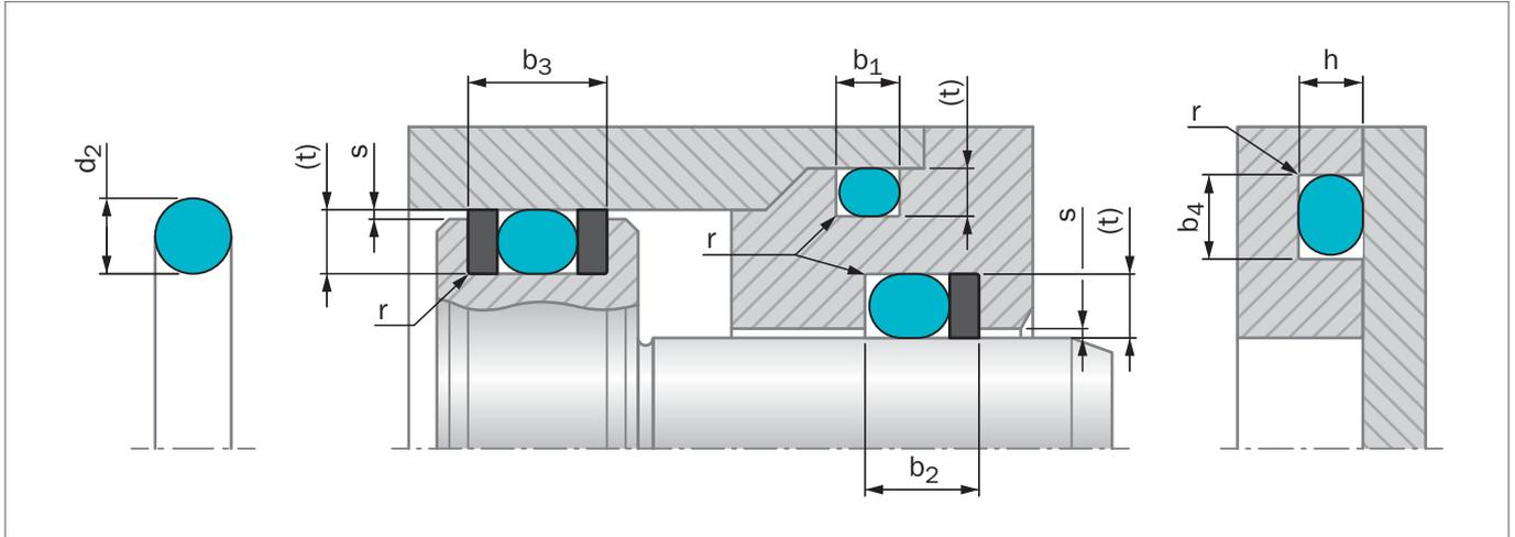
Figure 27: Installation drawing
