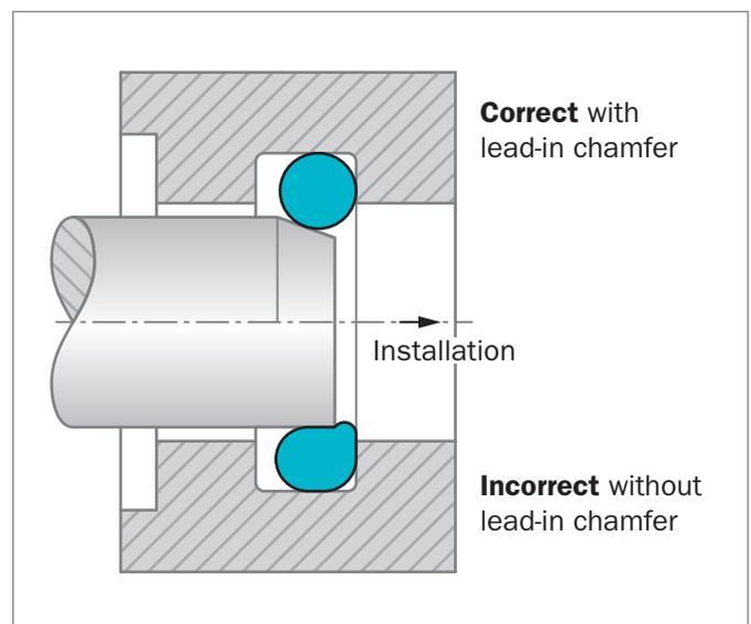
Figure 13: Rod installation with O-Ring
