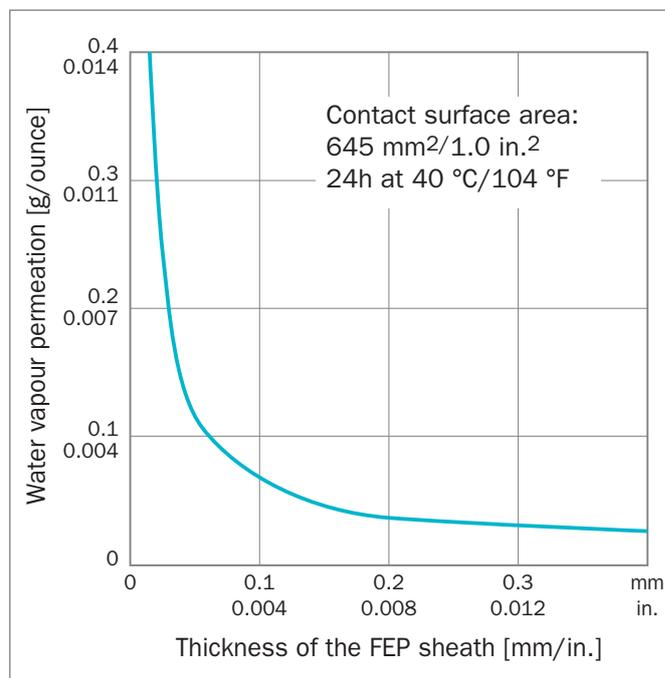
Figure 37: Water vapor permeation for FEP O-Rings
