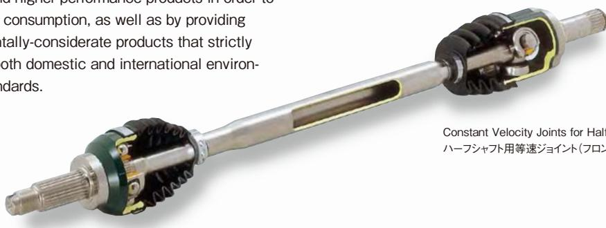
Constant Velocity Joints for Halfshaft
