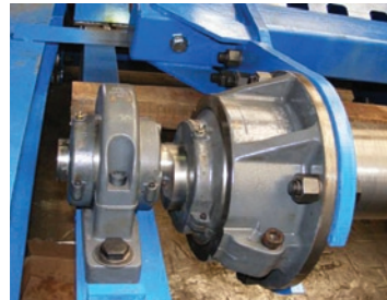
A Cooper square flange bearing arrangement in the dusty environment on a grain elevator
