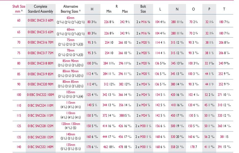
Metric Sizes Shown in Red. Imperial Sizes Shown in Black. Add EX to reference for Expansion Type or GR for Fixed Type. \* Shaft Size indicates standard SNC bearing. \* Alternative Bearing Sizes shown may be fitted in the same pedestal.
