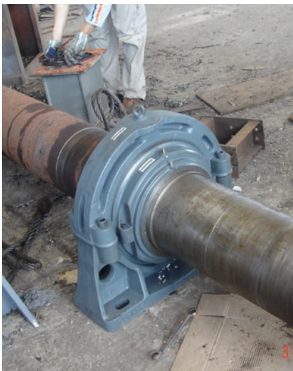
Cooper bearing during build-up of a new machine
