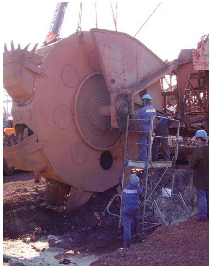
Typical stacker reclaimer bucket wheel during inspection for potential bearing conversion
